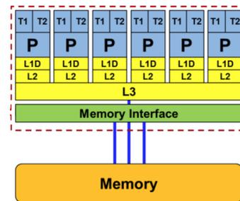
Figure 1: Memory hierarchy of a multicore architecture.
